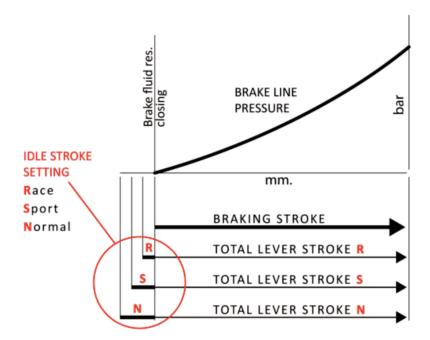
The effective (efficient) lever stroke is the total lever travel - to produce a certain pressure in the brake circuit- minus the idle stroke that is the distance between the main seal of the piston in neutral position and the inlet hole of the brake fluid (coming from the reservoir).
